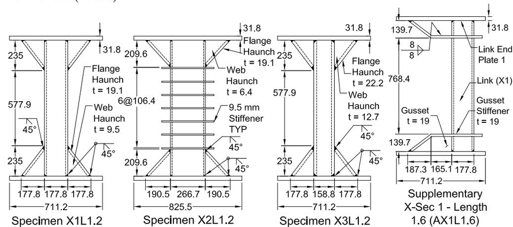
Figure 3. Example Link Specimen Elevations
